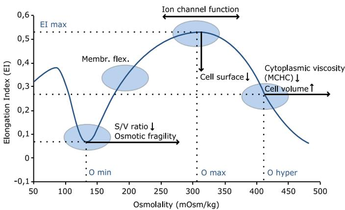
Fig. 5: With the Osmoscan 4 parameters are defined: *Omin* (osmolality at *Elmin*, hypotonic region), *Elmax* (maximal EI of the total curve), *Omax* (osmolality at *Elmax*) and *Ohyper* (osmolality corresponding to 50% of the *Elmax*; hypertonic region).
