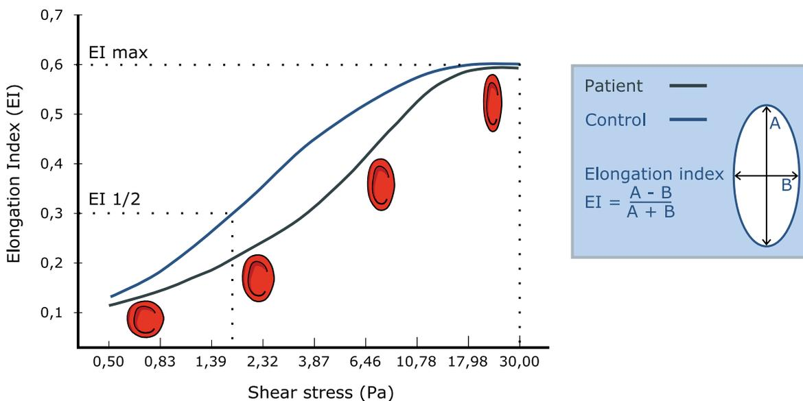
Fig. 3: Change in Elongation Index (EI) with applied shear stress; Parameterization of deformability curve.
