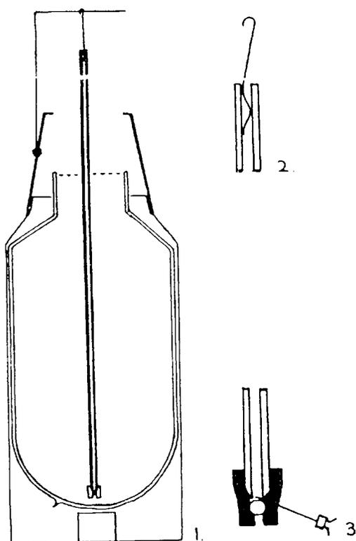
FIG. 1-1 Selection of "thermos" flask showing tube suspended in water. 2. Method of hanging tubes. 3. Method of sealing lower end of tube showing position of needle for filling.
